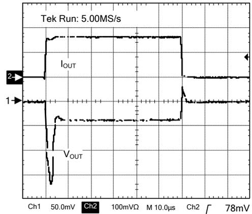
$V_{OUT}=2.5V$ ,  $I_{OUT}=50mA$ , no  $C_{IN}$ ,  $C_{OUT}=4.7\mu F$ ,  $t_s=t_f=20ns$
