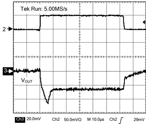
$V_{OUT}=2.5V$ ,  $I_{OUT}=0\sim 50mA$ , no  $C_{IN}$ ,  $C_{OUT}=10\mu F$ ,  $t_s=t_f=2ns$
