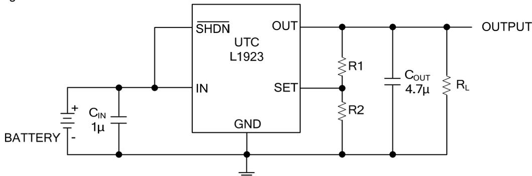
Figure 2. Adjustable Output Using External Feedback Resistors
