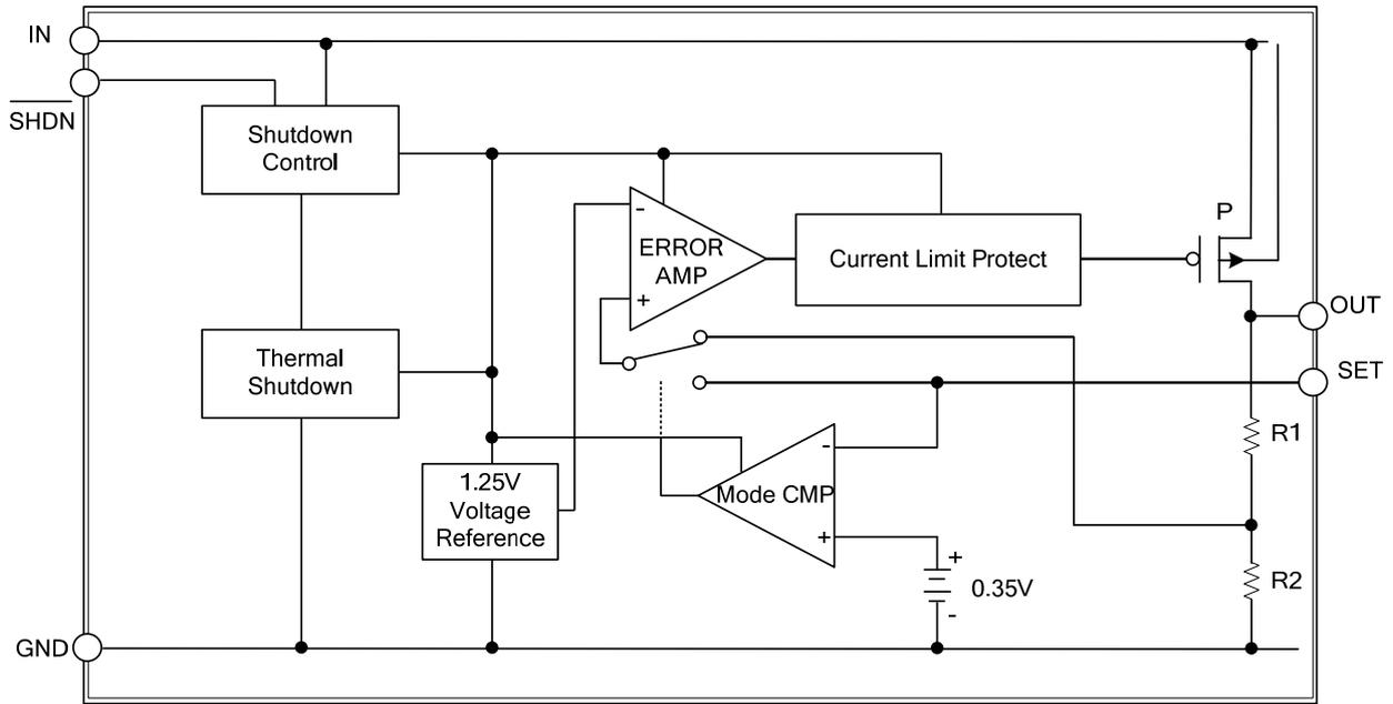
Fig.1 Functional Diagram
