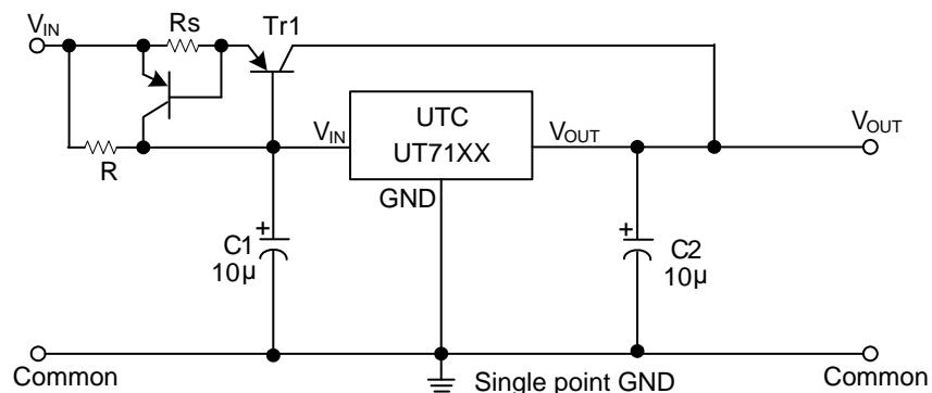
Circuit for increasing output voltage
