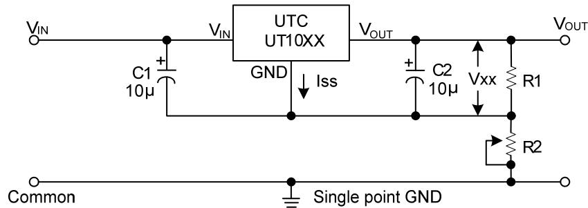
$$V_{OUT} = V_{xx}(1 + \frac{R2}{R1}) + I_{ss}R2$$
