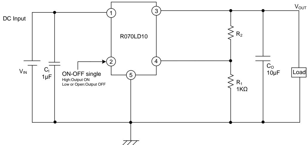
Note: There is no oscillation when both  $C_{IN}$  and  $C_{OUT}$  are removed, if applications are properly matched.
