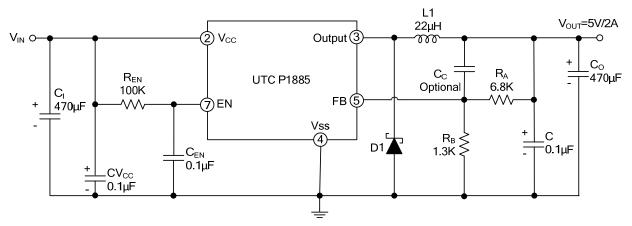
Note:  $V_{OUT} = V_{FB} x (1+R_A/R_B)$ ,  $R_B=0.7K^{\sim}5K$  ohm
