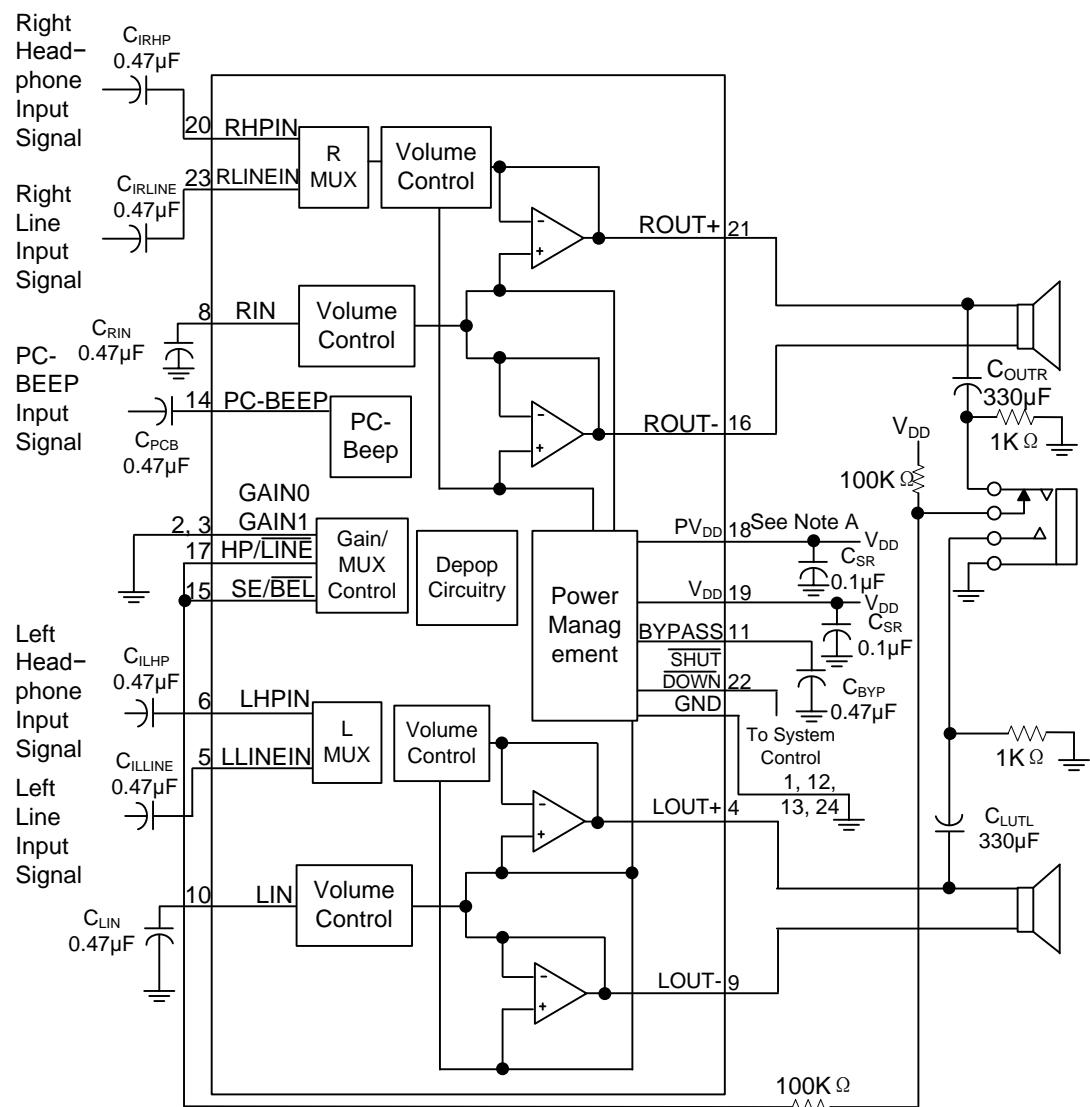
A. A 0.1-µF ceramic capacitor should be placed as close as possible to the IC. For filtering lower frequency noise signals, a larger electrolytic capacitor of 10 µF or greater should be placed near the audio power amplifier.
