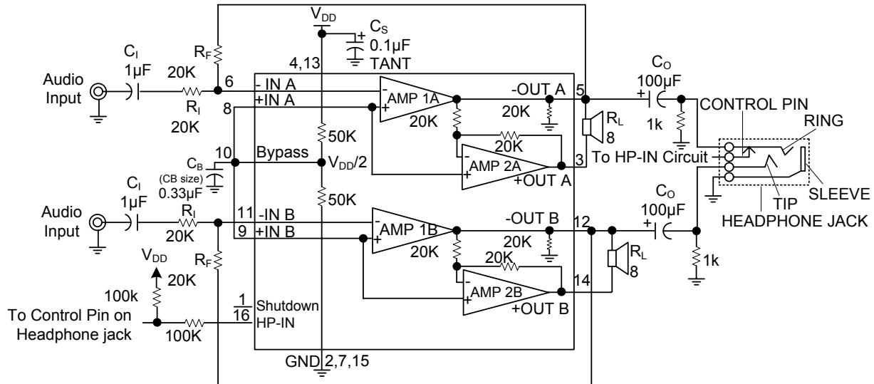
Note: Pin out shown for DIP-16 and SOP-16 packages. Refer to the PIN CONFIGURATION for the pin out of other packages.
