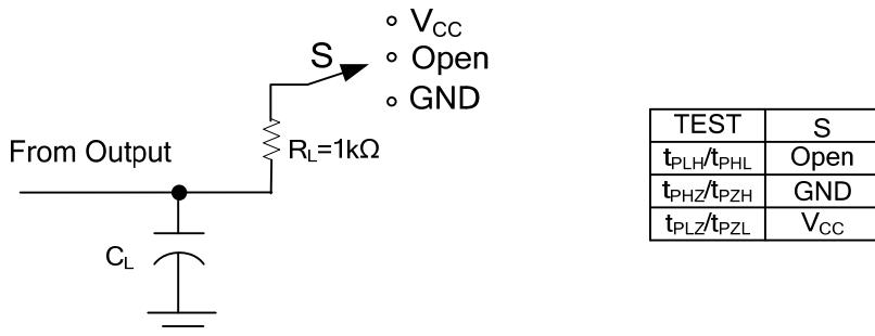
Test circuit for measuring propagation delay
