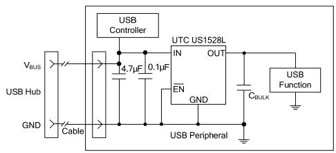
Figure 3. Inrush current-Limit Application
