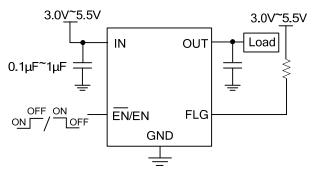
Figure 1. Supply Bypassing
