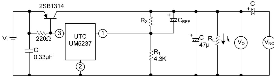
(b) Ripple rejection test circuit
