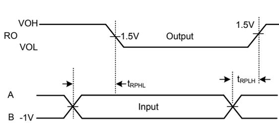
Fig. 9 Receiver Propagation Delays
