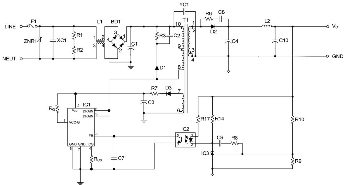
Fig.7 UTC UCS1652S Typical Application Circuit
