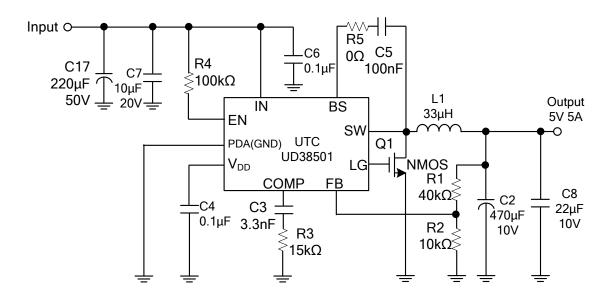
$V_{OUT}$ = $V_{FB}$  × (1+R1/R2),  $V_{FB}$ = 1.00V, R2 suggest 10k $^{\sim}$ 30k $\Omega$
