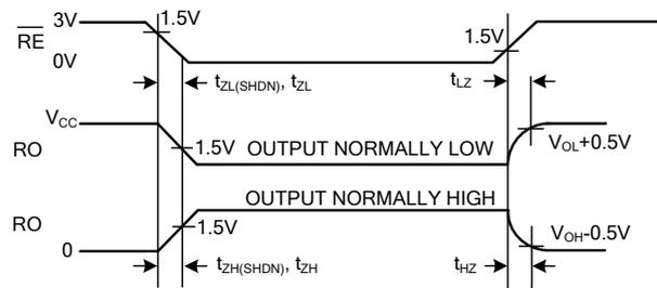
Fig. 8 Receiver Enable and Disable Times
