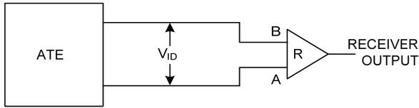
Fig. 9 Receiver Propagation Delay Test Circuit
