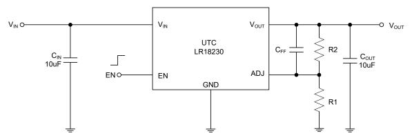
Cff option notes: the capacitance of feed-forward capacitor with range of 10pF to 1uF allows to achieve better PSRR performance when required by the application
