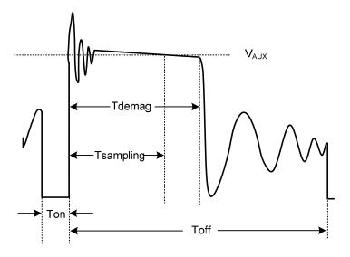
Figure 2. Auxiliary voltage waveform
