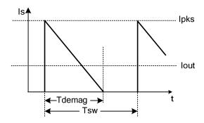
Figure 4. Secondary current waveform
