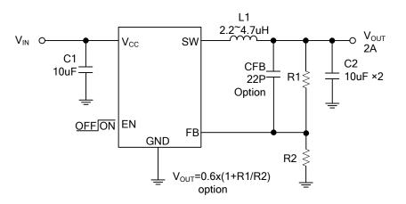
$V_{OUT}=V_{FB} \times (1+R1/R2), V_{FB}=0.6V, R2 suggest 60k^{300k}\Omega$
