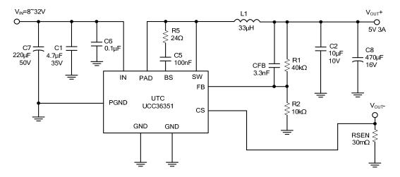
Note:  $V_{OUT} = V_{FB} \times (1 + R1/R2)$ ,  $V_{FB} = 1.00V$ , R2 suggest  $10k^{\sim}40K\Omega$ ,  $I_{SEN} = 3.3A$  ( $I_{SEN} = V_{CS}$  (0.1V)/RSEN (30m $\Omega$ )
