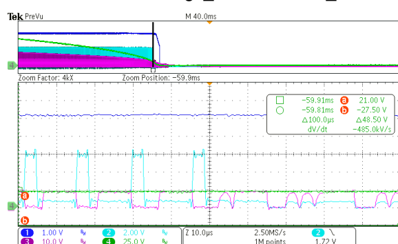
Fig. 39 90Vac/60Hz → AC OFF; 5V; 0.5A
