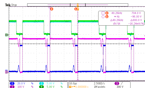
Fig.130 230Vac/50Hz; 5V; 100% Load, Ch1: SR MOS Drain. Ch2: SR MOS Gate. Ch3: Q1 Vds. Ch4: SR IC VG.
