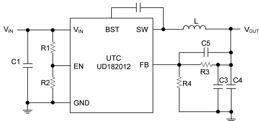
$$V_{FB} = V_{OUT} \times \frac{R4}{R4+R3}$$
