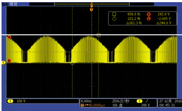
Fig3.VDS waveform@90Vac FULL LOAD
