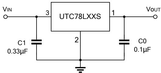
Notes: 1. To specify an output voltage, substitute voltage value for "XX".
