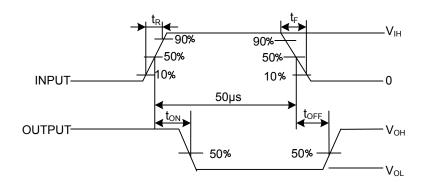
Notes: 1. Pulse width 50µs, duty cycle 10%, Output impedance 50 $\Omega$ , t<sub>R</sub> ≤ 5ns, t<sub>F</sub> ≤ 10ns. 2. See below.
