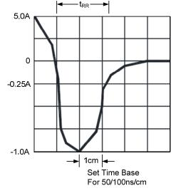
Notes: 1.Rise Time=7ns Max. Input Impedance=1 megohm. 22pF 2.Rise Time=10ns Max. Source Impedance= $50\Omega$
