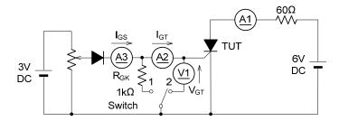
Switch 1:  $I_{GT}$  measurement. Switch 2:  $V_{GT}$  measurement
